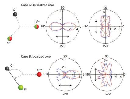
Polar plots of molecular-frame photoelectron angular distributions obtained after photoionization of  $CS_2$  10 eV above the S 1s threshold from different kinematical conditions. Ref) R. Guillemin et al., Nat. Comm. 6 (2015) 6166.
