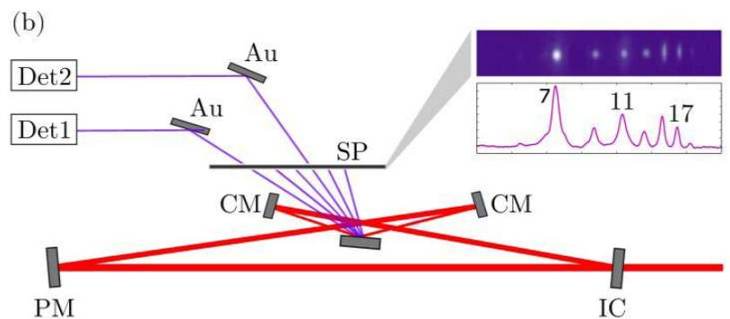
Figure 1: Femtosecond enhancement cavity with input coupler (IC), plane mirror (PM), two curved mirrors (CM), sodium salicylate plate (SP) and two gold mirrors (Au). The harmonics are out-coupled from the cavity via a combined reflector/diffraction grating. Harmonic 11 and 17 are optionally sent through apertures in the SP to independent detectors (Det1 and 2).
