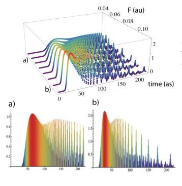
Figure description: Tunneling time probability distribution calculated in the context of strong field ionisation using the path integral approach. Top: distribution at different field strengths, Panel a: F=0.04 au; Panel b: F=0.1 au
