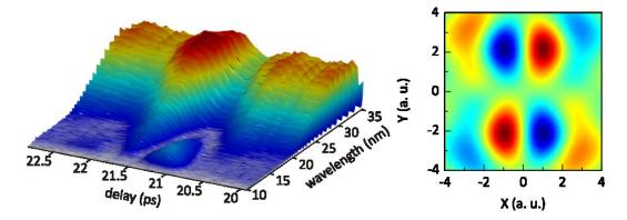
A macroscopic ensemble of molecules exposed to an intense laser pulse emits coherent XUV radiation appearing as high-order harmonics of the laser frequency. The spectral amplitude and phase of the radiation produced by single molecules is encoded in the macroscopic emission. Molecular imaging by high-order harmonics [1] requires the measurement in amplitude and phase of the harmonic field emitted by a single molecule for different molecular orientations.
