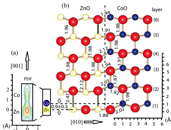
Fig.1: (a): Probability density function of the (Zn,Co) site in the first Zn(Co) O layer next to the Ag(111) surface. Maxima are related to Zn and Co. Boxes indicate different size scale between (a) and the structure model in (b). Wurtzite-type CoO is separated from h-BN-type ZnO. The vertical line indicates the phase boundary. Distances are given in Å, and layers are labeled from (1), next to the Ag(111) surface to (6). (taken from H.L. Meyerheim et al., PRL 102, 156102 (2009))
